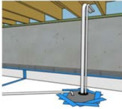
Figure 25. Crock pit lid sealing
