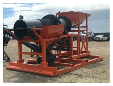
The introduction of hydro-vac slurry to the trommel.
