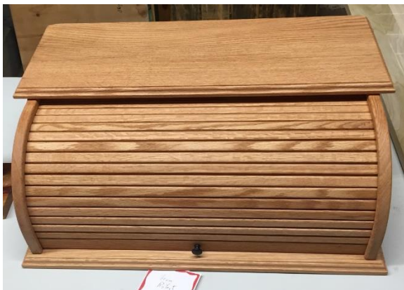
Vern Rotert; Oak breadbox with tambour door. He used a ball and socket router bit set to make the door.
