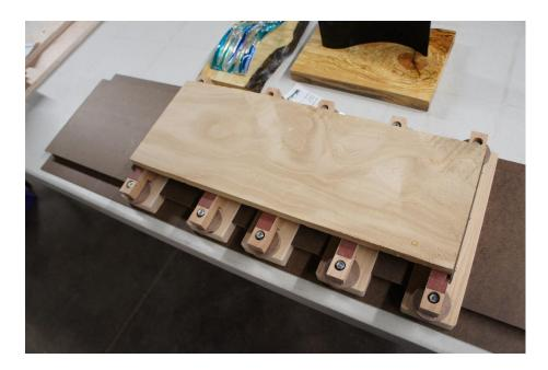
This last show and tell project is a planer leveling jig made by Vern Rotert. It is a design made from a Woodsmith weekend project. It is used to flatten twisted or otherwise uneven boards. The bars beneath the work piece are adjustable giving support to the piece can be ran through a thickness planer, flattening one side. This is great for those boards that are too wide to face joint on your jointer, or if you don't have a jointer this would be faster than flattening by hand.
