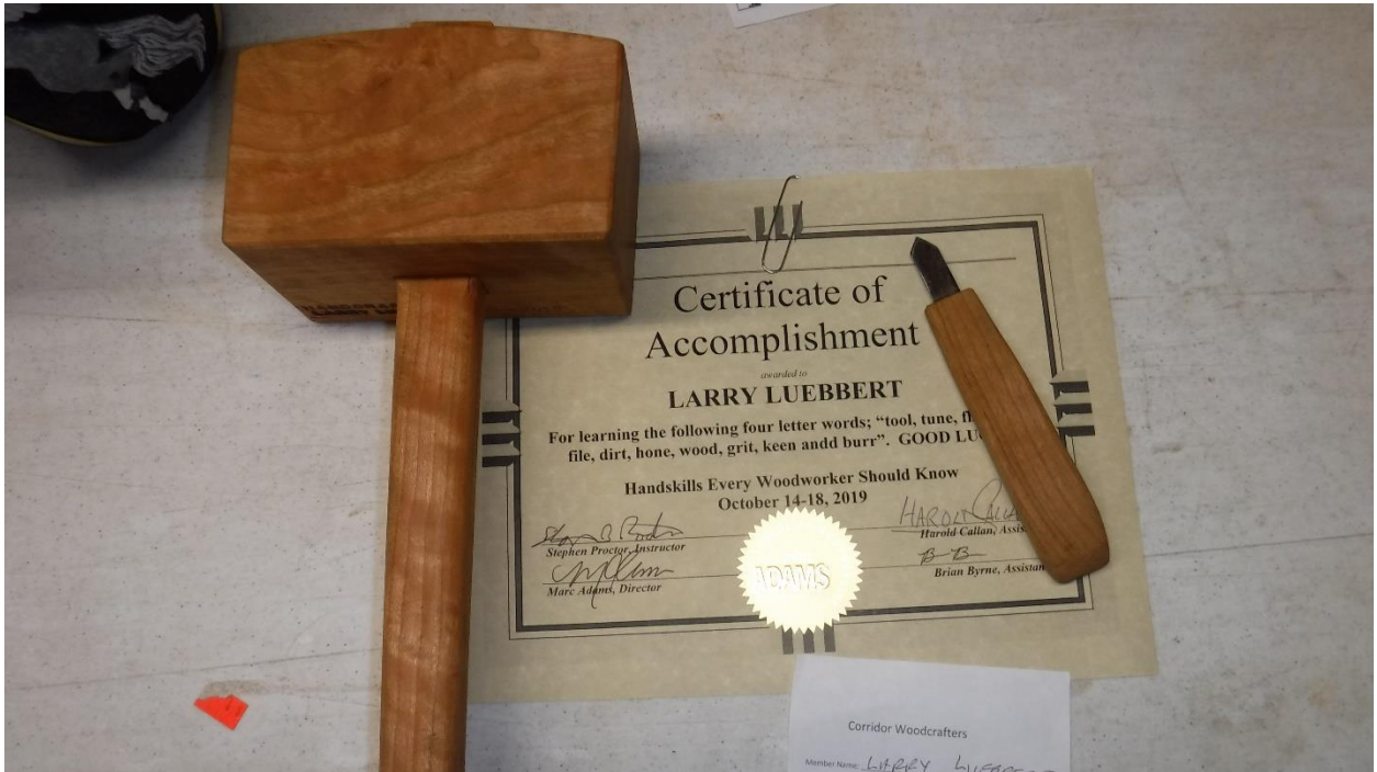
Larry Lubbert attended a Hand Skills every woodworker should know class given at the Marc Adams School of Woodworking in Indiana, taught by Steve Proctor. The Marking knife and mallet were hand made by him at the school out of cherry. The blade for the marking knife is made from a hacksaw blade. Good job Larry.
