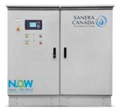
These generators use a special hydraulic configuration to produce Anolyte using less salt and energy. Brine flows through the anodic chamber and a small amount of water through the cathodic chamber. This configuration use a 0.15% brine concentration as the precursor. The pH of the Anolyte is similar to the pH of the soft water used in the production of anolyte but can be regulated as low as ~ 5.5 by including additional components during the generator build.
