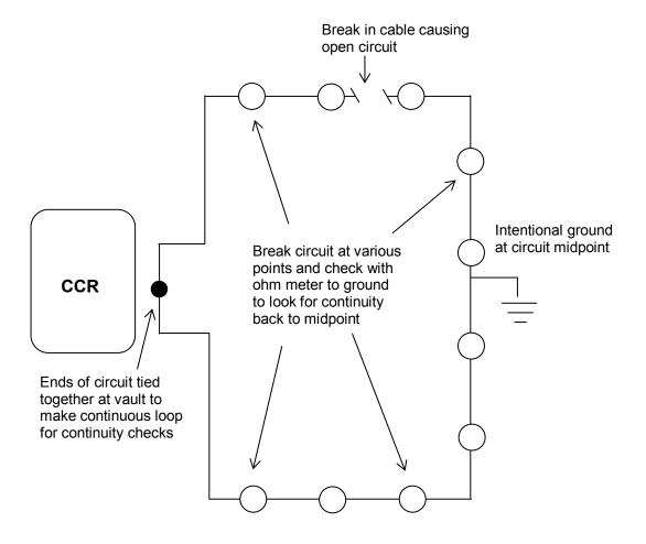
Figure 6-5. Locating Open Circuit Faults
