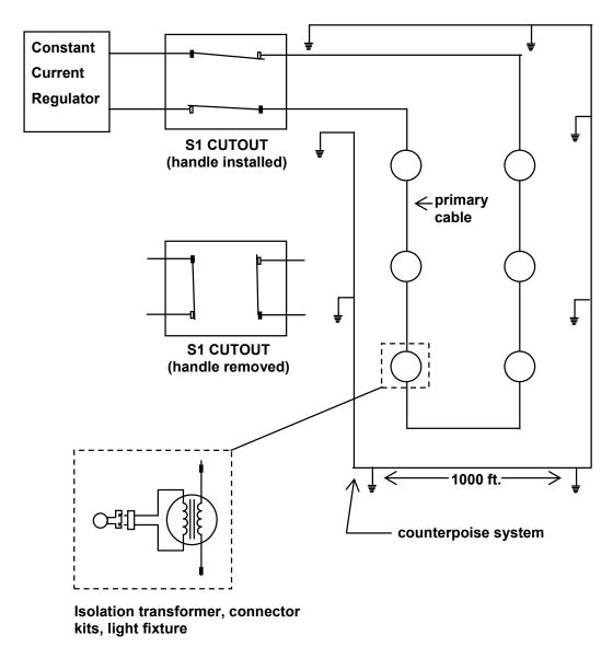
Figure 6-1. Typical Series Lighting Circuit
