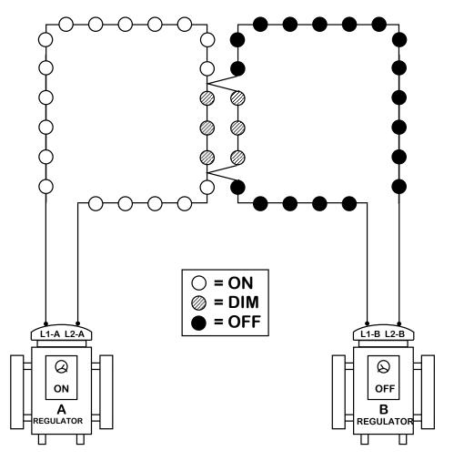
THIS CONDITION CAN BE DETECTED BY OHMMETER TESTING RESISTANCE BETWEEN LOAD "A" AND LOAD "B."
