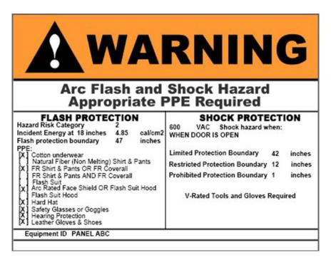
Figure 2-1. An Arc Flash Warning sign
