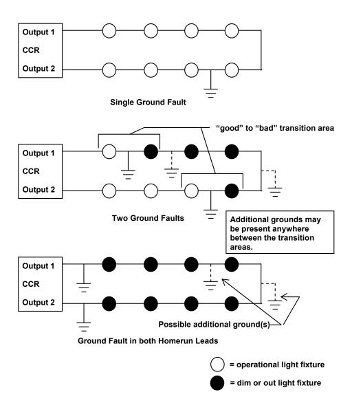
Figure 6-2. Typical Ground Faults
