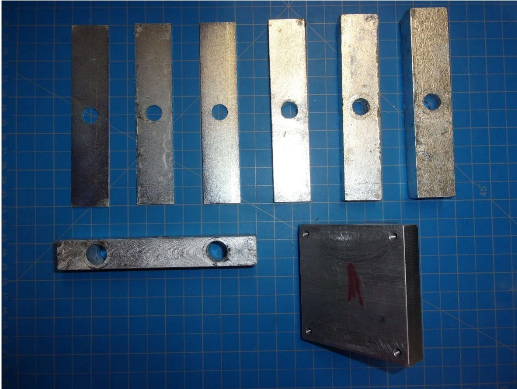
HDG (Galvanized) Samples: Spacers – (1) 3/4"; (1) 1/2"; (1) 1/4"; (1) 1/8"; (2) 1/16" Impact Plate and Mounting Bar
