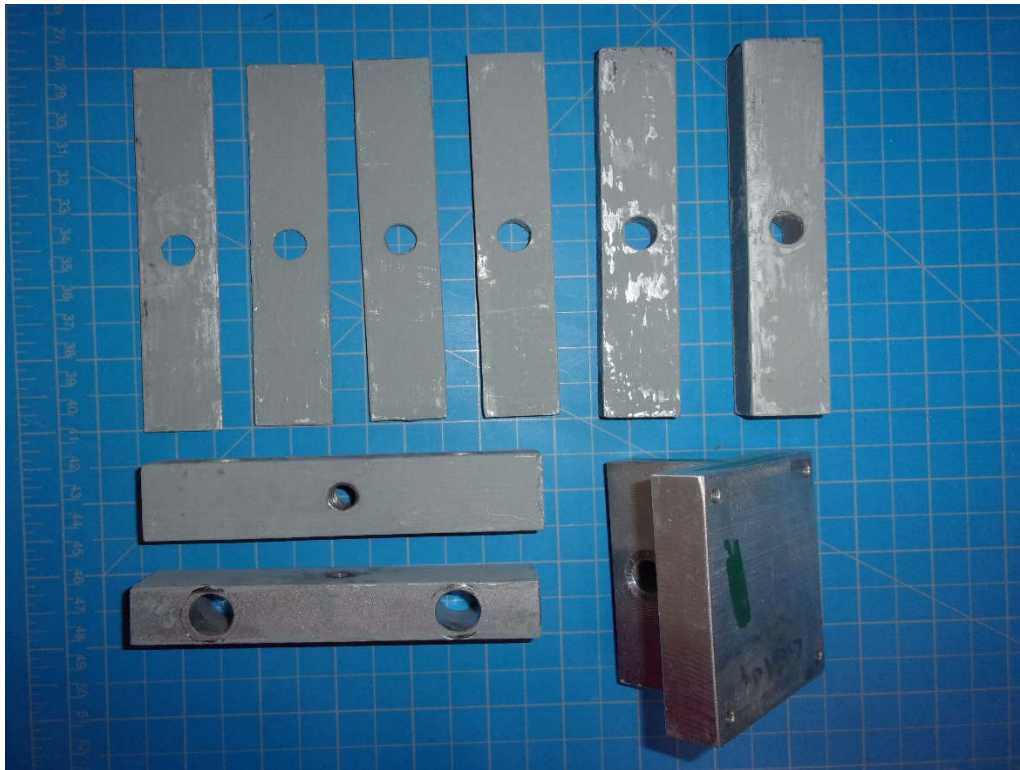
B50 (RCSC Class B Coating) Samples: Spacers – (1) 3/4"; (1) 1/2"; (1) 1/4"; (1) 1/8"; (2) 1/16" Impact Plate and Mounting Bars
