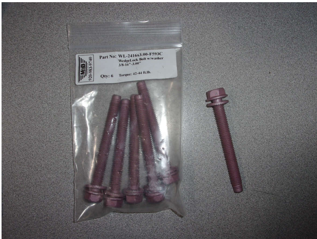
DUT Test Bolts (SAE J429 Grade 5 Bolt – Top and ASTM F593C Bolt – 3.00” – Bottom)
