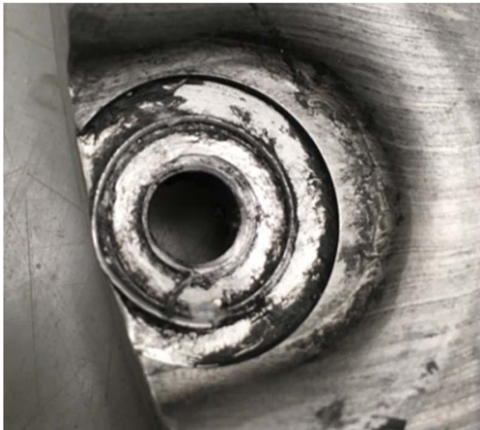
heavy machining and hole bulging - LSA
