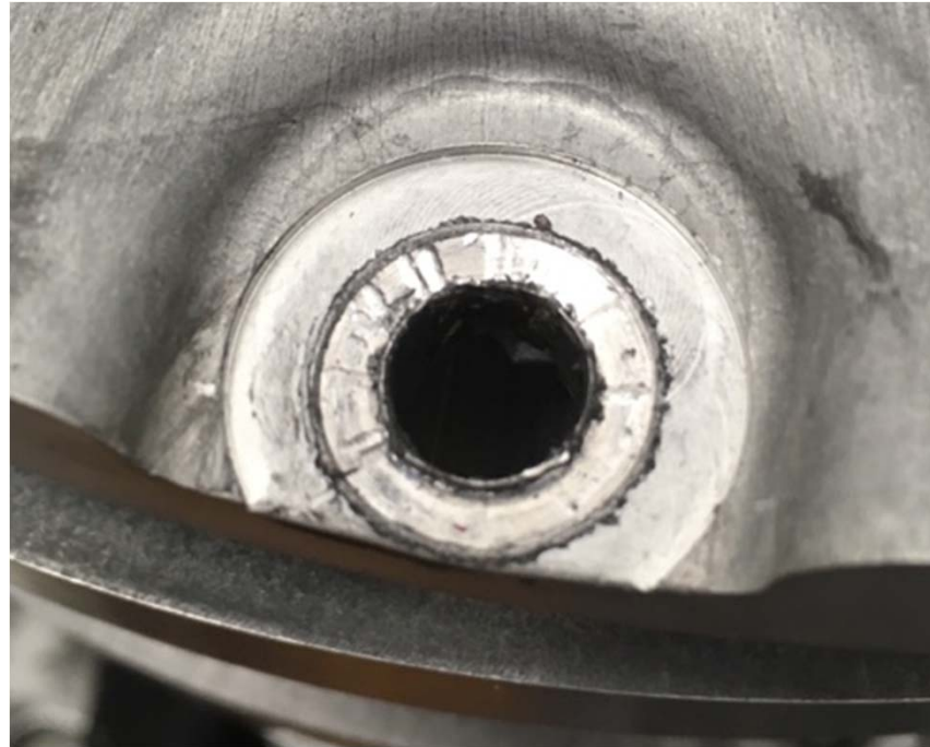
Light machining of bolt hole - LSA
