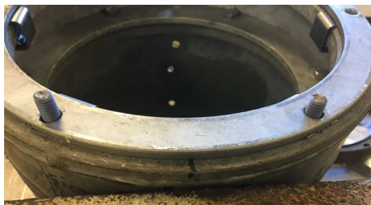
Disassembled fixture w/ broken bolts as found post test
