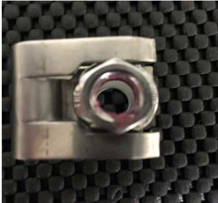
Noted that hex nut was found turned in clip after vibration testing
