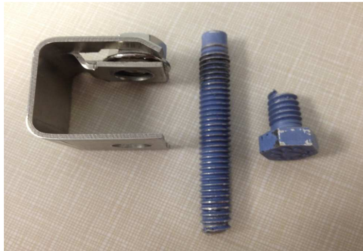
Clip, nut, and bolt after test
