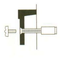
Expansion sleeves for mounting to brick, stone or cement with optional rosette covers (see below).
