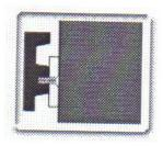
Letters are pre-mounted in the factory to an aluminum bar. For letters 6" in cap height and greater, we recommend using a double bar mount. Letters under 6" would normally use a single bar mount.
