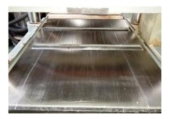
**ON A MORE SERIOUS MATTER:** Above right is a disappointing photo of the club's thicknesser which has received some abuse. It is obvious that something metallic has been embedded in wood that was put through the cutter resulting in deep gouges in the smooth surface of the plate. Please ensure that there are no **NAILS, SCREWS, STAPLES or STONES** in your wood before attempting to put it through the machine.
