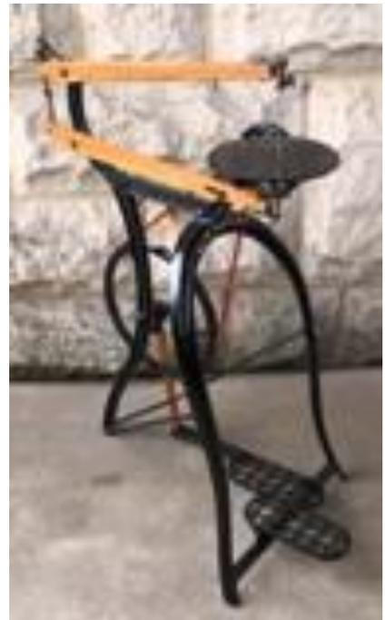
*available. A friend TIG welded the broken casting, I machined a spindle for the main pulley, re-manufactured part of the frame and sourced a belt. The top & bottom beams are timber as is the link from the treadle to the main pulley, these were all re-made at the Club.*
