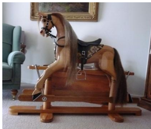
Pat Mahoney has finished the horse he was making for his wife, Sue. Pat says, "It is a number 3 size & is made from Karie, the swing frame is also Karie which came from a double bed frame. The mane & tail are horse hair & I used 4 coats of Hames clear varnish. The swing irons are 12mm stainless steel rod & where they fit through the hoof rails they pass through a 12mm ball race."
