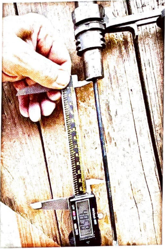
Plug guages used to observe wear progression in throat, bore, and muzzle.
