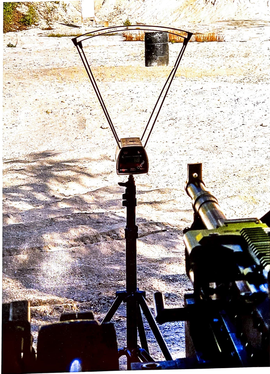
Test set-up at 100 meter range with chronograph.
