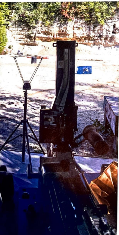
Muzzle velocity measured every 250 rounds.
