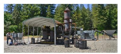
Pictured above is the pyrolysis operation run by the Redwood Forest Foundation in Piercy, California in 2017. Tan oak was harvested from overcrowded areas of the Usal Forest and converted to high-quality biochar, then sold into the local community as a soil amendment.
