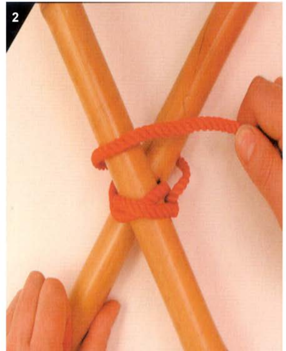
STEP TWO. MAKE A TURN AROUND THE TWO CROSSED POLES, PULLING THE TIMBER HITCH TIGHT.
