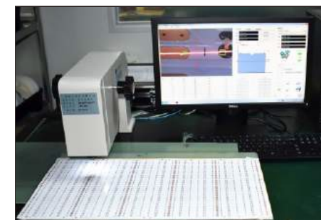
TIN THICKNESS TESTING
