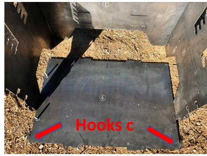
6.- Slide plate #4 and insert in bottom slots on plate # 1,#2,and#3, insert two linchpins to secure plates in place.
