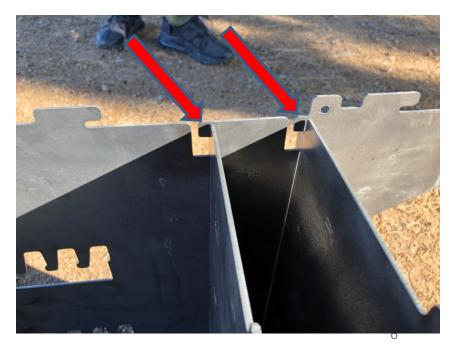
11.- Place plate #6 on the remaining side. Insert all the remaining linchpins (8 on the front and 2 on the back).
