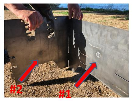
4.- Find plate #3 and insert it in right slots of plate #1 with numbers facing inside the assembly, insert two linchpins to secure plates in place.
