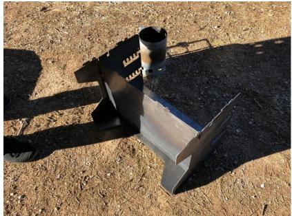
9.- Find plate #5 and insert it in the remaining slots on plates #1,#2, and #3 as shown on the top right picture.
