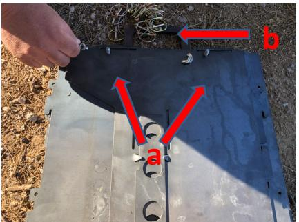
3.- Find plate #1 and #2. Insert plate #2 on left slots of plate #1 with numbers facing inside the assembly, insert two linchpins to secure plates in place.
