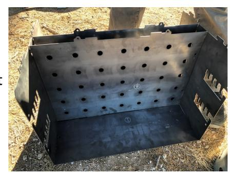
10.-Make sure that the front of plate #4 and #5 are touching the bottom side of slots on plates #2 and #3 to receive plate #6.
