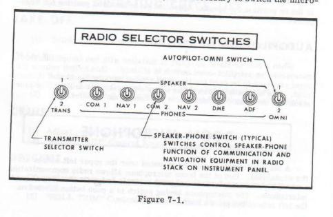
phone to the radio unit the pilot desires to use for transmission. This is accomplished by placing the transmitter selector switch in the position corresponding to the radio unit which is to be used. The up position selects the upper transmitter and the down position selects the lower transmitter.
