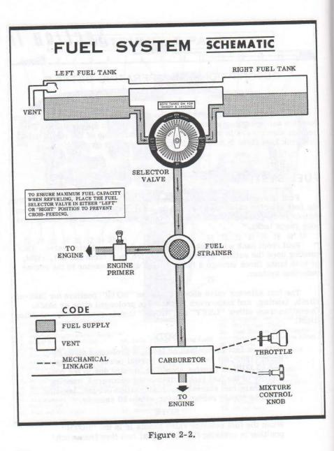
tank may occur if the wings are not maintained exactly level. Resulting wing heaviness can be alleviated gradually by turning the selector valve handle to the tank in the "heavy" wing.
