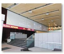
Plank: T&G grid clip, T&G direct attach clip Panel: Z-bar/Z-clip, torsion spring
