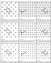
The Fusion line of acoustic wall panels features wood veneer with a variety of perforation options. Standard perforations are available in 6mm or 8mm diameter holes in 16mm or 32mm on-center spacing. Square and diamond perforation patterns, custom diameter, spacing and other patterns are available, as are slotted perforations. Wall panels install with traditional Z-clips. For projects requiring sound absorption, recycled cotton acoustical backer can be installed behind the Fusion wall panels.
