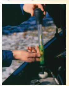
**Hydrometers** A hydrometer is a device that measures the specific gravity (the ratio of the fluid's density to that of water) of a fluid. Fluids of different densities result in different readings. Hydrometers are often used at service stations to diagnose problems with an automobile's battery.
