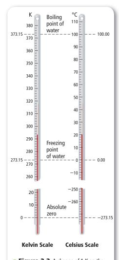
■ **Figure 2.3** A change of 1 K on the Kelvin scale is equal in size to a change of 1°C on the Celsius scale. Notice also that the degree sign (°) is not used with the Kelvin scale.
