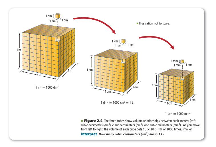
For smaller quantities of liquids in the laboratory, volume is often measured in cubic centimeters (cm<sup>3</sup>) or milliliters (mL). A milliliter and a cubic centimeter are equal in size.
