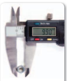
**Figure 2.11** This digital caliper is being used to check the size of a nut to one-hundredth of a millimeter (0.01 mm). Skill is required to correctly position the part in the caliper. Experienced machinists will obtain more precise and more accurate readings than inexperienced machinists...
