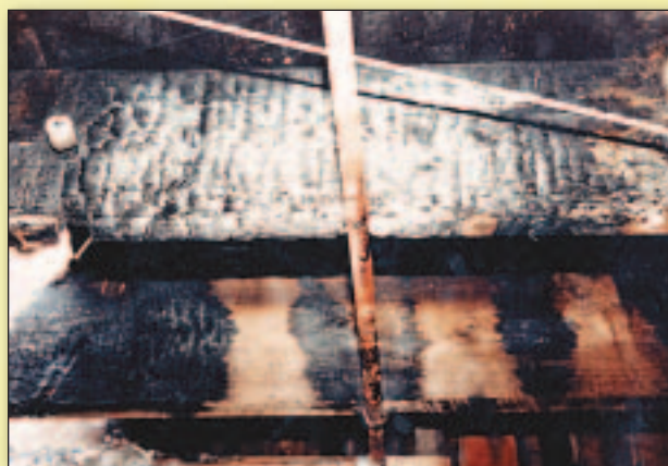
Figure 1 Accelerants can cause a rundown burn pattern.
