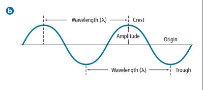
■ **Figure 5.3** These waves illustrate the relationship between wavelength and frequency. As wavelength increases, frequency decreases.
