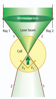
**Figure 1** As the laser passes through the cell, the beam is bent. The cell feels a force in the opposite direction of bending and so is held within the beam of light.
