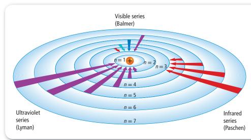
■ **Figure 5.11** When an electron drops from a higher-energy orbit to a lower-energy orbit, a photon is emitted. The ultraviolet (Lyman), visible (Balmer), and infrared (Paschen) series correspond to electrons dropping to n = 1, n = 2, and n = 3, respectively.
