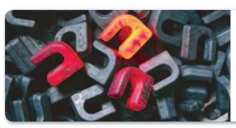
**Figure 5.6** The wavelength of the light emitted by heated metal, such as the iron at left, depends on the temperature. At room temperature, iron is gray. When heated, it first turns red, then glowing orange.
