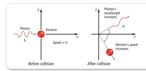
**Figure 5.14** When a photon interacts with an electron at rest, both the velocity and the position of the electron are modified. This illustrates the Heisenberg uncertainty principle. It is impossible to know at the same time the position and the velocity of a particle.
