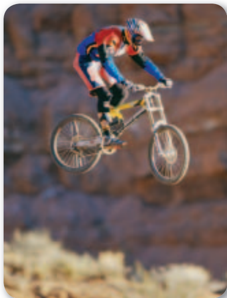
■ Figure 7.13 Bicycle frames are sometimes made of 3/2.5 titanium alloy, an alloy of titanium containing 3% aluminum and 2.5% vanadium.
