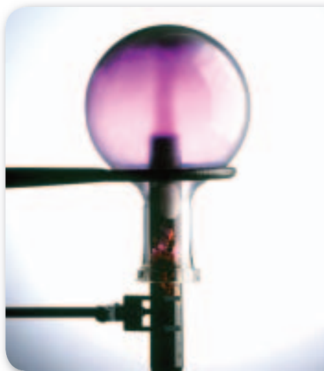
■ Figure 7.3 When zinc reacts with iodine, the heat of the reaction causes solid iodine to sublime into a purple vapor. At the bottom of the tube, ZnI_2 is formed containing Zn^{2+} ions with a pseudo-noble gas configuration.
