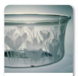
■ Figure 8.6 The frosted-looking portions of this glass were chemically etched using hydrogen fluoride (HF), a weak acid. Hydrogen fluoride reacts with silica, the major component of glass, and forms gaseous silicon tetrafluoride (SiF<sub>4</sub>) and water.
