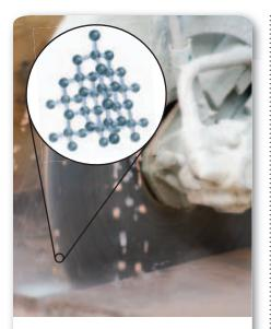
■ Figure 8.25 Network solids are often used in cutting tools because of their extreme hardness. Here, a diamond-tipped saw blade cuts through stone.
