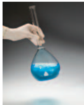
Step 2: The solute is placed in a volumetric flask of the correct volume.
