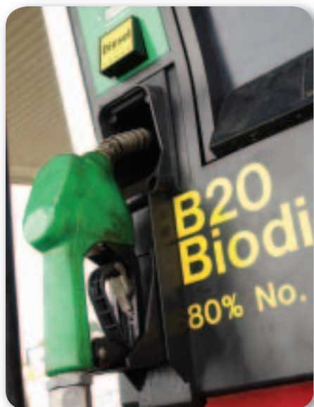
■ Figure 14.5 B20 is 20% by volume biodiesel and 80% by volume petroleum diesel. Biodiesel is an alternative fuel that can be produced from renewable resources, such as vegetable oil.
