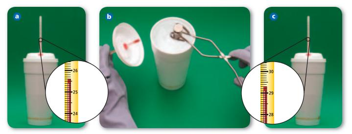
■ **Figure 15.6 a.** An initial temperature of 25.60°C is recorded for the 125 g of water in the calorimeter. **b.** A 50.0-g sample of an unknown metal is heated to 115.0°C and placed in the calorimeter. **c.** The metal transfers heat to the water until metal and water are at the same temperature. The final temperature is 29.30°C.
