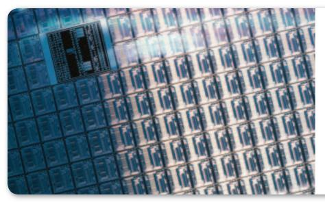
**Figure 15.16** Sulfur hexafluoride is used to etch minute and sometimes intricate patterns on silicon wafers in the production semiconductor devices. Semiconductors are important components of modern electronic equipment, including computers, cell phones, and MP3 players.
