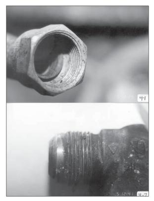
Figure 3 - Kitchen Range Flexible Connector Mating Fittings as Found after Explosion Even
