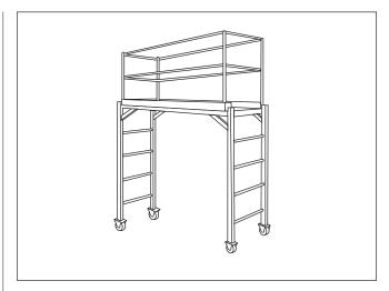
Fig. 3: Manually Propelled Scaffold
