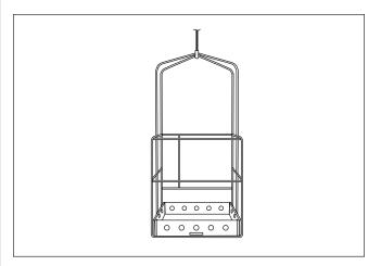
Fig. 4: Single-Point Suspension Scaffold
