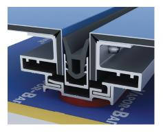
ECONECT-GS<sup>™</sup> metal composite panel system relies on a hard silicone gasket to provide protection from the water intrusion. This design offers a more elegant appearance than the more common wet-caulk systems. In case of panel damage, replacement of the panel is possible thanks to the removable gasket design.
