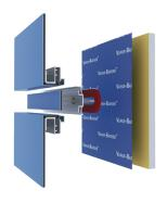
As a rainscreen type panel system, it must be installed onto an already waterproofed wall surface. An array of shims can be used to correct for wall variations and insure perfect panel system flatness. ECONECT-RS™ system is designed to channel rain water down through special weep holes, which are located on the bottom horizontal edge of each panel.
