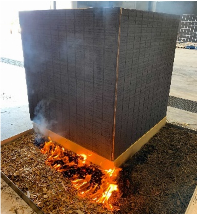
Figure 4. Exterior wall exposed to a small fire with 6-in noncombustible vertical clearance.
