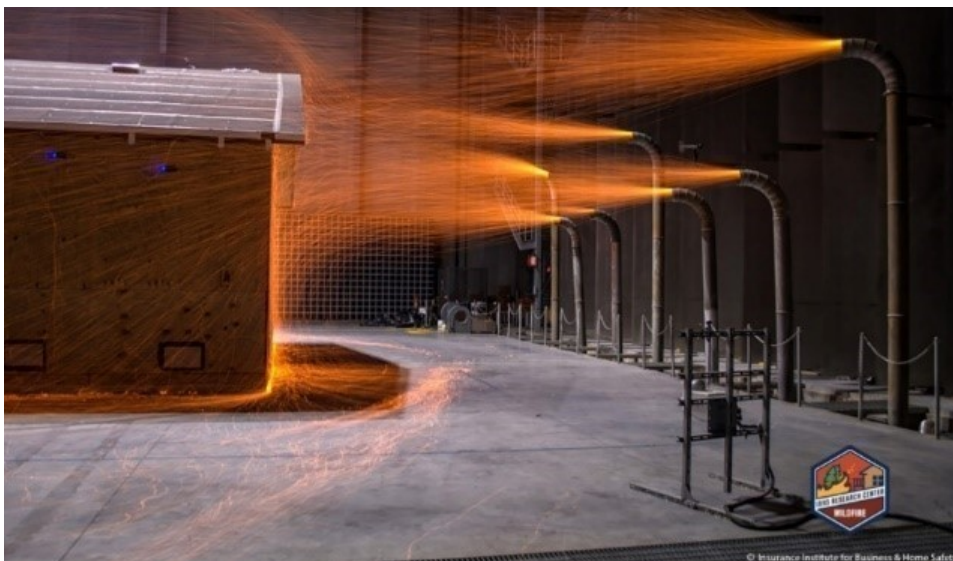
Accumulation of embers at the base of the exterior wall.
