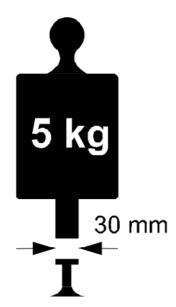
The device used to measure the thickness of clothing and shoes must be capable of measuring to one-tenth of a millimeter (0.1 mm). Measurements must be taken with a 5.0 kg weight applied. The device must have two (2) circular flat surfaces facing each other, each 30 mm in diameter.
