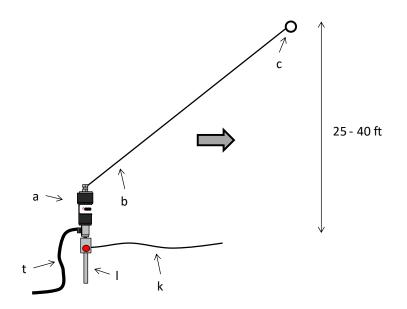
Figure 4. Sloping Wire Configuration.
