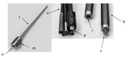
Plate 4. Whip Antenna and Spike Mount Connections.
