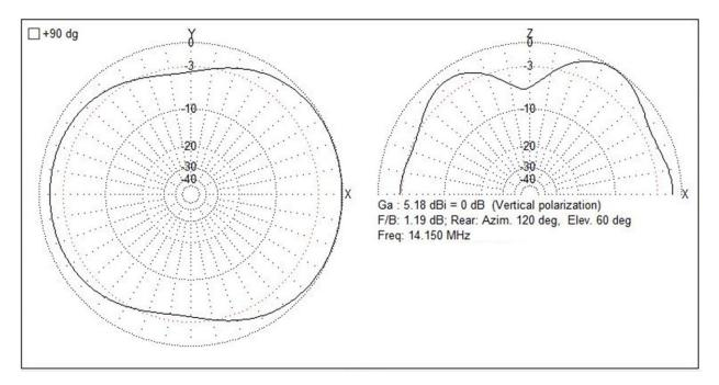
Figure 13. Sloping Wire Far Field Plot 14 MHz.
