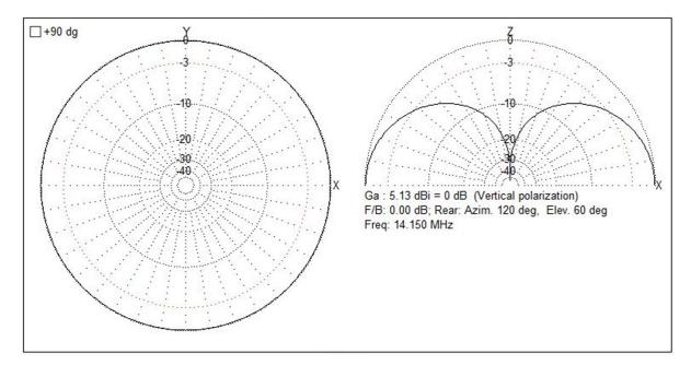
Figure 11. Portable Vertical Far Field Plot 14 MHz.
