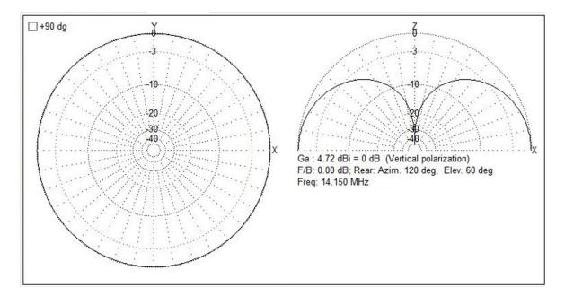
Figure 10. Manpack Vertical Far Field Plot 14 MHz.
