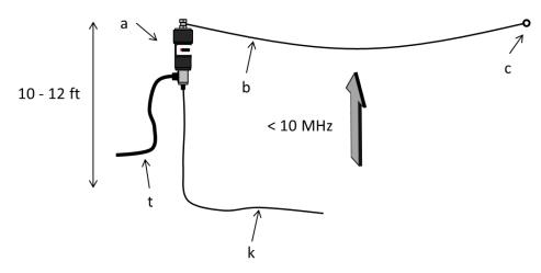
Figure 3. Horizontal NVIS Configuration.
