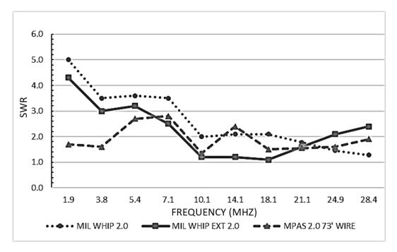
Figure 9. SWR by Frequency Graph.
