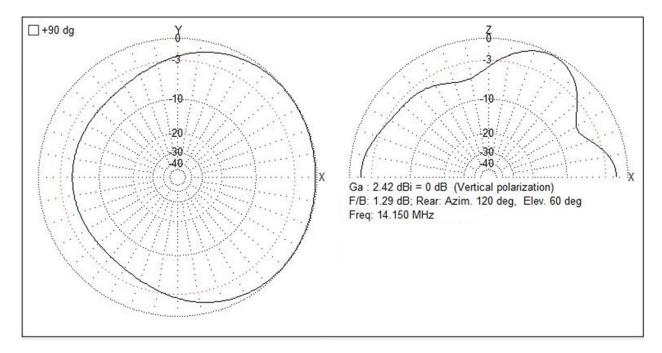
Figure 14. Inverted "L" Far Field Plot 14 MHz.
