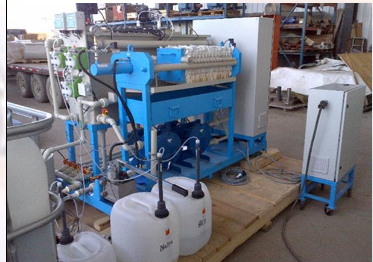
ClearBLUE™ miniflot 5 m3/day (up to 50,000 m3/day per unit)
