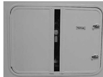
The Propane Tank Compartment Door provides access to the storage propane tank(s) and regulator valve(s). This compartment door must remain unlocked as required by National Fire Protection Association (NFPA) to allow immediate access in case of a propane leak or fire. A large red propane label is located on the door to aid emergency personnel to rapidly locate the gas valve.
