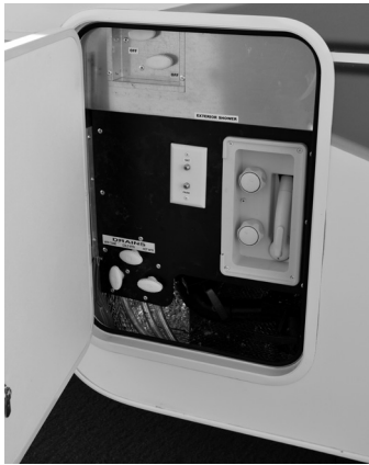
The Exterior Service Center Door provides access to waste tank dump valves, fresh water drain and winterizing valves.
