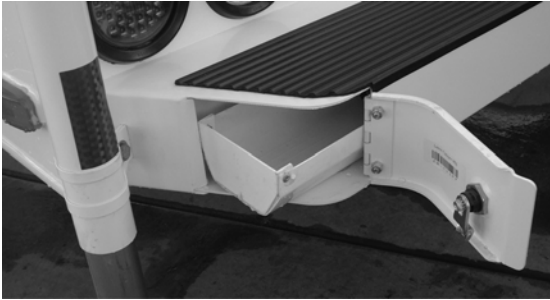
The Bumper Hinged Door provides storage and convenient access to the waste drain hose and storage tray.
