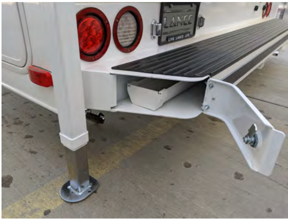
The Bumper Hinged Door provides storage and convenient access to the waste drain hose and storage tray.
