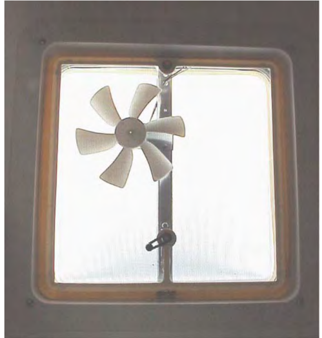
The roof vents are operated from inside and have built-in screens. To operate, turn the crank in the center of the vent clockwise to open and adjust. The bath vent may be equipped with a 12-volt exhaust fan. The switch to control the fan is located on the vent. These vents may be left slightly open while traveling, but be careful when traveling where vertical clearance is limited. Vent lids can crack if left open too far.
