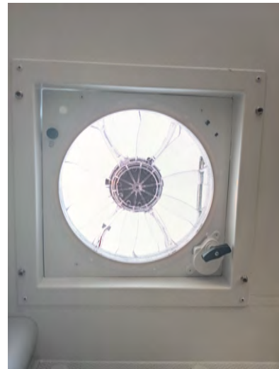
The Fantastic high-volume power roof vent is designed to quickly exhaust stale hot air. Some models are equipped with a reversing fan that will also draw in fresh air. Due to the proximity of holding tank vents located on the roof, some models do not have this feature.
