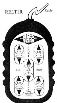
NOTE: THE BUTTONS ON THE TRANSMITTER FUNCTION AS FOLLOWS: THE "UP" ARROW SIGNIFIES LIFT THE CAMPER, WHILE THE "DOWN" ARROW MEANS LOWER THE CAMPER.
