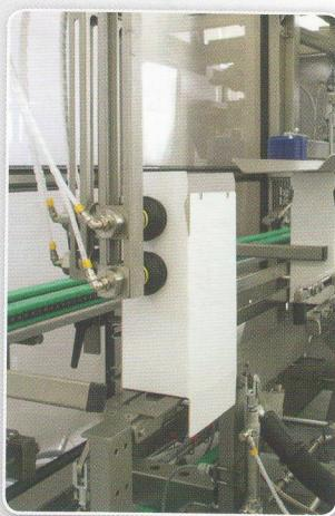
Automatic box erector with closing of the lower flaps by means of Hot Melt glue
