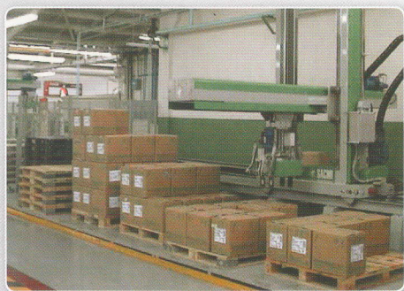
Cartesian coordinate robot with maximum pallet height of 2400 mm
