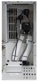
3. Working from left to right, disconnect the cables and then the hoses.
