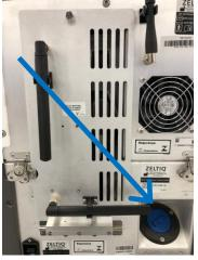
2. Press down on the recessed end of the blue lever on the chiller tank cap.
