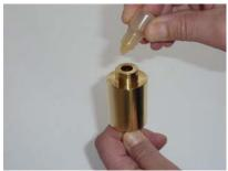
8. Making sure you do not lose the thrust ball, carefully lower the bronze housing onto the bearing shaft while gentle rotating it back and forth to spread oil on all the bearing surfaces. Once fully home, spin the bearing six or more times with your thumb and forefinger to pump oil up into the top of the bearing. (The bearing pumps oil if spun clockwise only).
