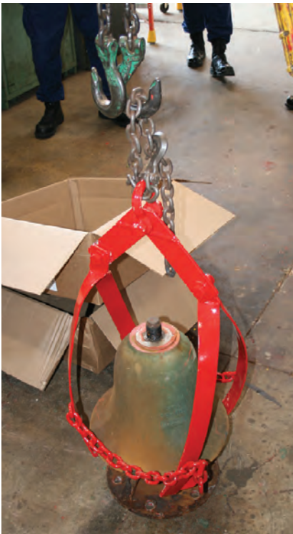
At left: The bridle for lifting a bell onto an aid.
