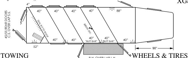
R.H. OVER LAP L.H. 2 5/16" ADJUSTABLE COUPLER (25,000# RATING) SAFETY CHAINS WITH SAFETY HOOK LATCHES
