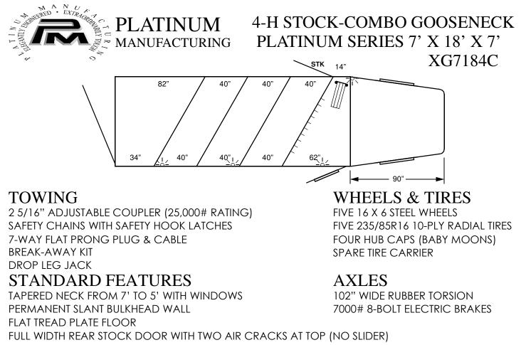
DRESSING ROOM DOOR (LINE) WITH WINDOW AND CAMPER LATCH WITH DEAD BOLT ESCAPE DOOR, (STANDARD STOCK TYPE) AT BULKHEAD, STREETSIDE WITH BUTTERFLY LATCH SINGLE SIDE WALL CONSTRUCTION, WITH TWO AIR CRACKS AT TOP IN HORSE COMPARTMENT AND SMOOTH SKIN AT TOP IN DRESSING ROOM AREA
